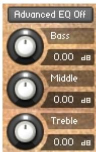
The EQ can either be a simple Bass/Middle/Treble Equalizer, with predefined Frequency and Bandwidth. Or an Advanced 3-Band Parametric Equalizer.
