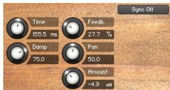
The **Feedback** knob sends a portion of the output back into the input of the delay line, which creates repeating echoes. A value of 0 produces only one echo, higher values give multiple echoes.
