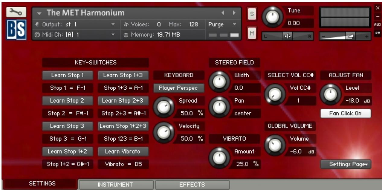
On the Settings Panel, you set the keys that will act as Key-Switches for the Stops and the various Stop combinations, and the Vibrato. You can control the Keyboards Perspective, Spread and Velocity. And also adjust the Stereo Field of the instrument, and control the Amount of the Vibrato. The CC# that will control the Volume can be selected, and the Global Volume adjusted. Finally you can set the Engine Fan Level and turn the fan button click On/Off.
