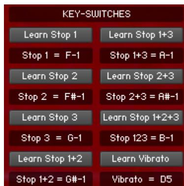
The Stop Label now shows the new note name of the Key-Switch, and the color code on the virtual keyboard updates to the selected key.
