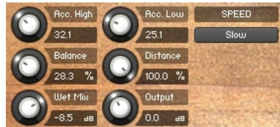
The **Balance** knob sets the ratio of the sound produced by the rotating speakers high frequency horn compared to the low frequency woofer. Higher values produce more highs, lower values more bass.
