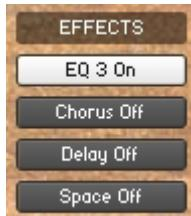
The four Effect buttons turn the various Effects On and Off, and opens the corresponding Page.
