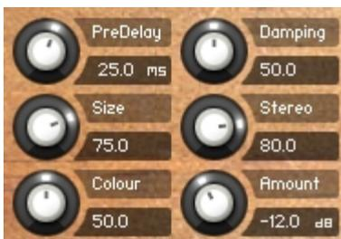
The **Predelay** knob introduces a short amount of delay before the reverb takes effect. Increase this parameter to simulate larger rooms, decrease it for smaller rooms.
