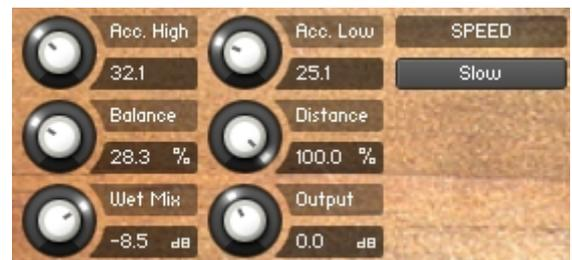
The **Distance** knob edits the distance between the virtual microphones and the rotating speaker. Higher values increase the distance.
