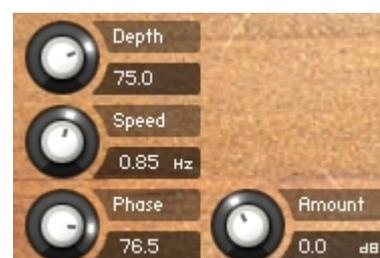
The **Phase** knob adjusts the phase difference between the two LFOs that drive the left and right stereo channels.
